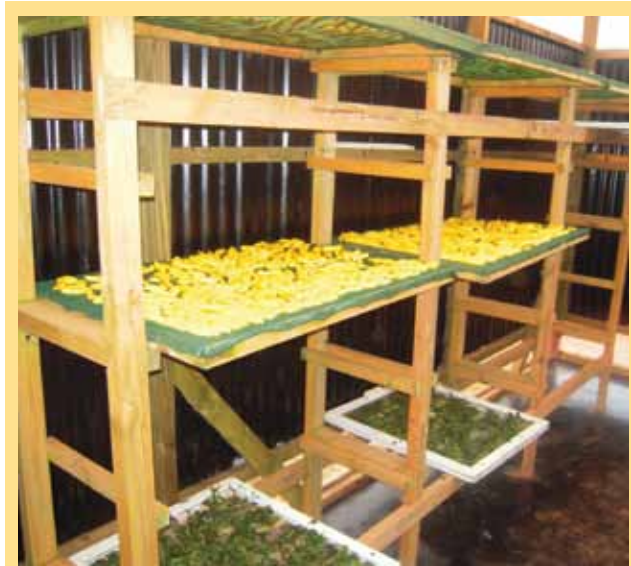
Drying in progress inside a walk in solar drier—these driers are being promoted
