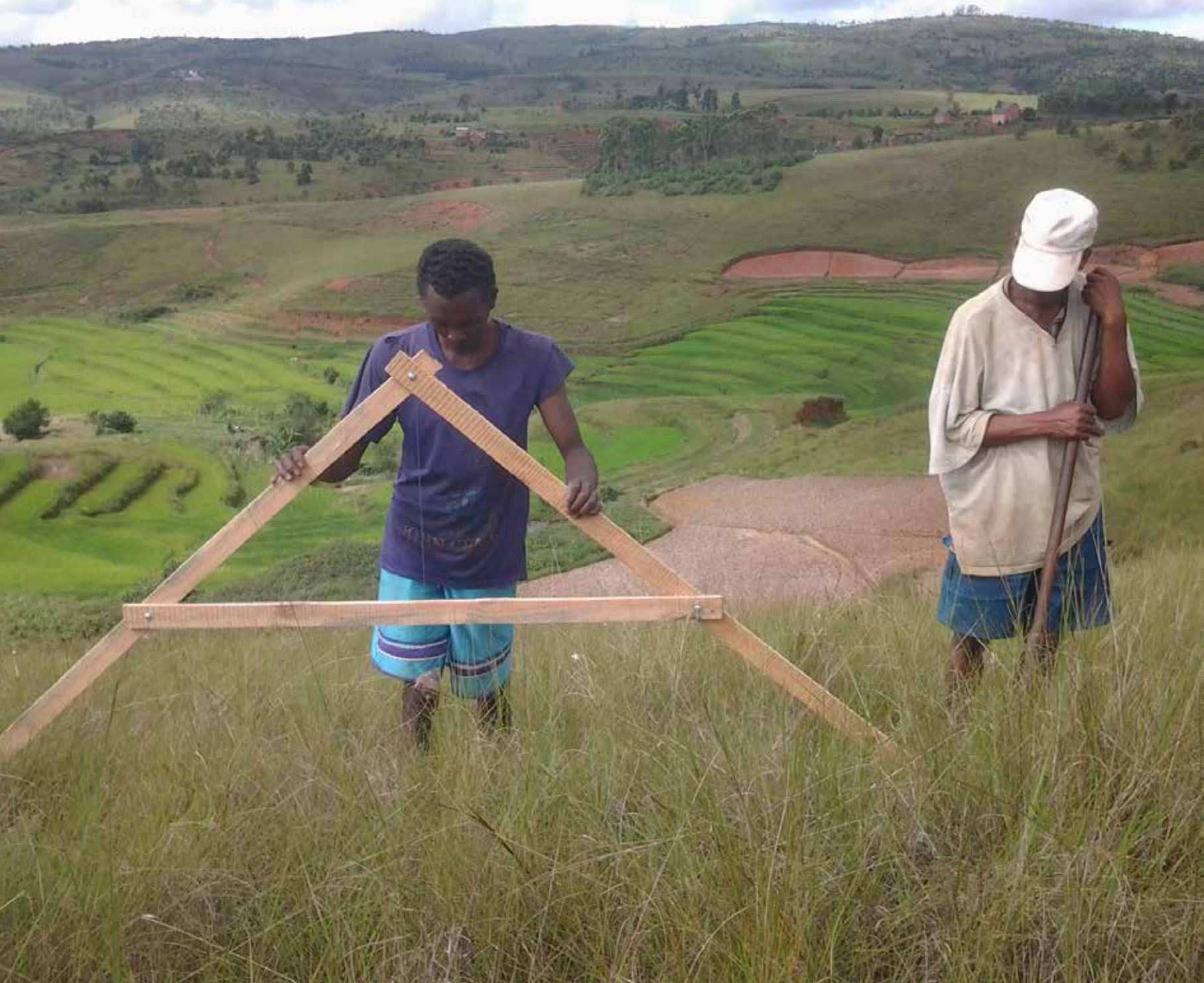
Youth in Madagascar use a locally fabricated tool to map contour lines. The lines are crucial in planning water and soil management activities such as landscaping, construction of terraces and water benches etc.
