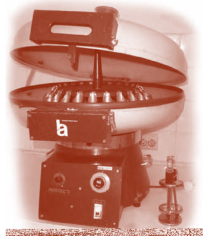
Kifaa cha kupimia mafuta cha Gerber
